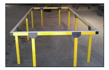
**Coast Mountain Bus Company** in Vancouver, BC uses FRP railing for their elevating platforms on the trucks used to maintain electric trolley wires. As FRP does dot conduct electricity, it provides a strong, safe alternative to steel or aluminum.
